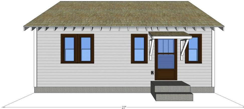
Figure 8: Measured drawing of north elevation of Assistant Ranger Dwelling.
